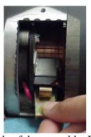
Pull the brush out of the slot and leave it hanging by the side of the assembly. Repeat this step for the brush on the other side of the motor. Never perform this procedure with the brushes still in their holders.
