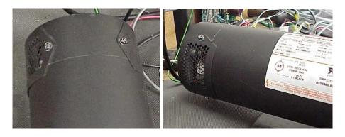
Place one of the brushes back into its slot and replace the clip that holds it in place. Repeat this step for the brush on the other side of the motor. The contour of the brush <u>must</u> match the contour of the motor, or the brush will not make proper contact with the commutator.
