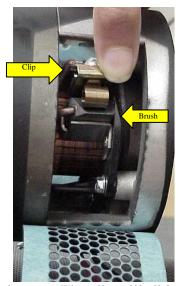
Push the clip in and towards the brush to free the catch on the bottom. The clip will slide out.
